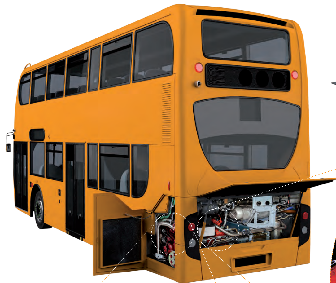
RS Oil Replenishment System with Remote Fill
